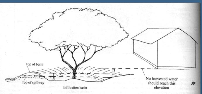
Fig. 1.12. Three important elevations: Elevation 1: Overflow spillway is the low point of earthwork's perimeter. Elevation 2: Spillway is low enough to ensure nothing is accidentally flooded. Elevation 3: Basin is lower than elevation of spillway to ensure water is harvested, rather than drained.
