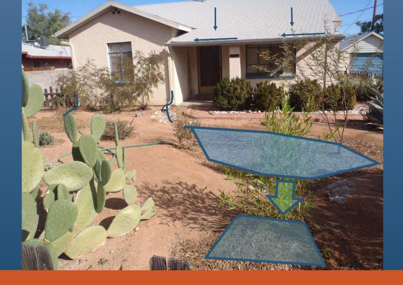
4. Spread and infiltrate the flow of water Water Harvesting Principles
