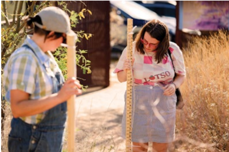
Marci Pullen learns how to use a bunyip, a simple water level that can be used to measure slope and grade changes to construct basins and swales.
