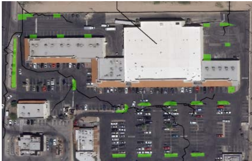
Figure 9. Example of GSI features in parking lots and open space at a school. Black lines represent flow lines in the flow accumulation layer.
