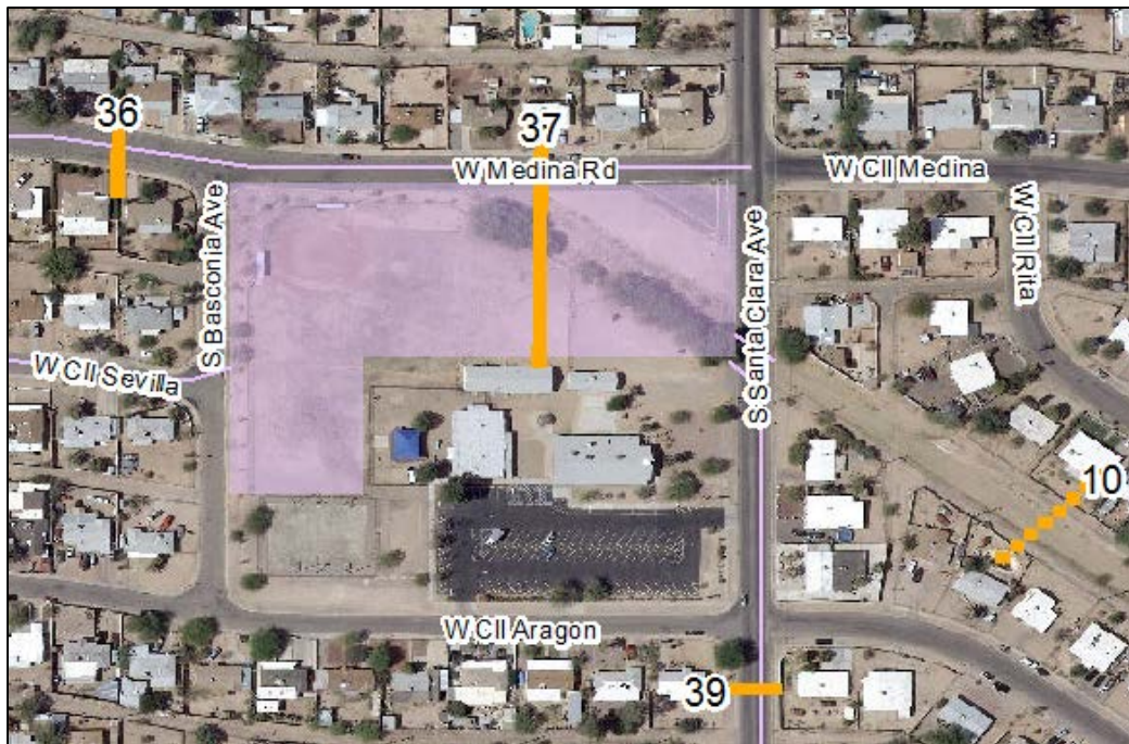
Figure 16. Hope United Methodist Church proposed grey infrastructure (purple) with model cross section locations shown in orange.
