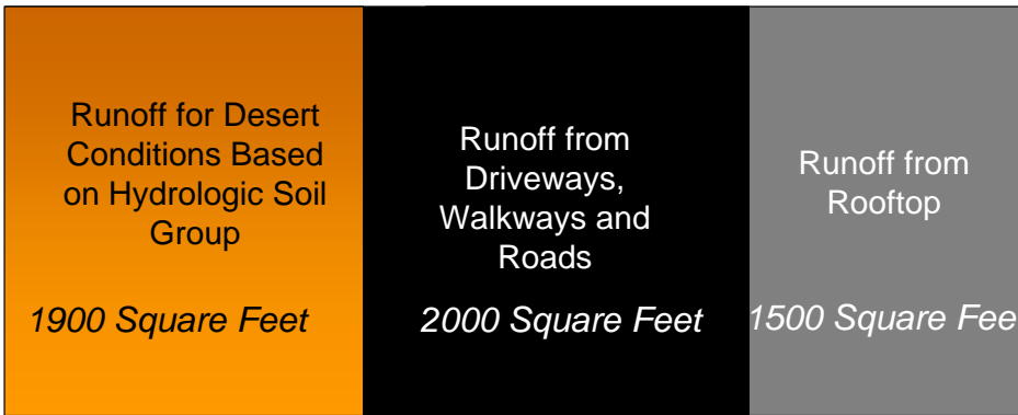
Figure 3b – Schematic of runoff conditions following development. Runoff increases because of impermeable rooftops driveways and other surfaces
