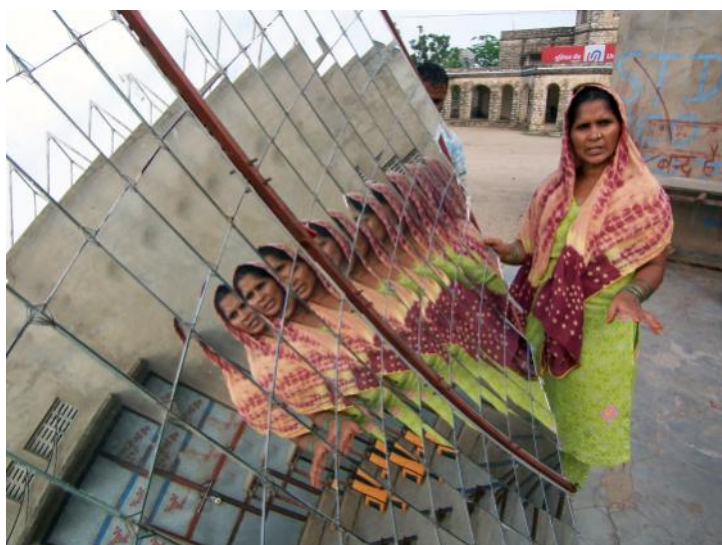
A "barefoot solar engineer" explains a parabolic solar cooker in Tilonia, Rajasthan
